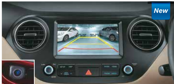
Rear Parking Assist System (with display on 17.64 cm Audio Screen)
